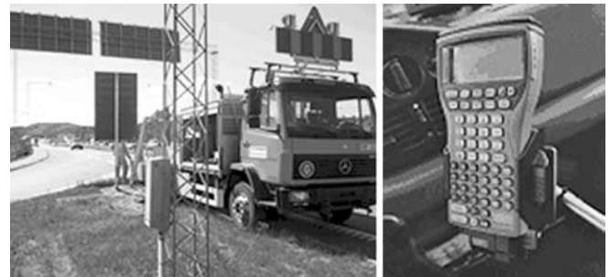
Fig. 1 Road inspectors taking care of a defective road sign (left). The current reporting-system used by the road inspectors (right)
